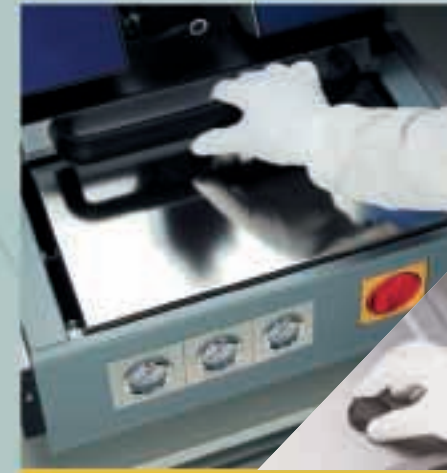
Push sliding table under split-field camera of CCTV and carry out fine alignment.
