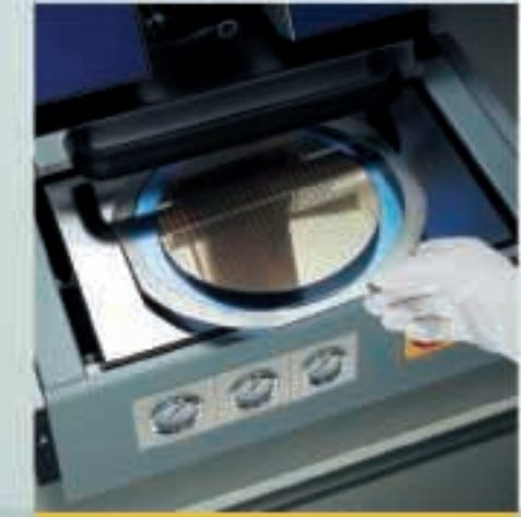
Push sliding table in again to mount new wafer and to remove wafer already mounted.
